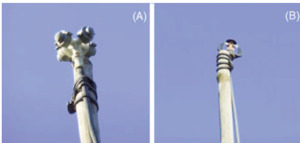
Figure 1. Overhead microsprinkler (A) and sprinkler (B) irrigation systems.
